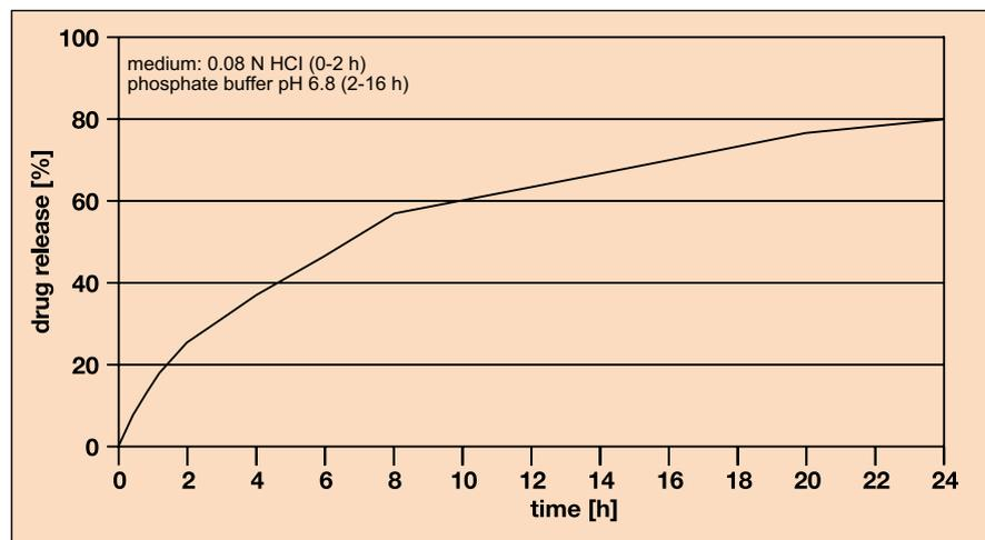
Fig. 8: Dissolution of Diclofenac sustained release tablets
