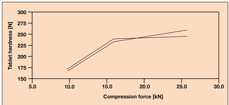
Fig. 4: Hardness-compression force profile of propranolol sustained release tablets containing 50% of Kollidon SR (2 Lots, Formulation see chapter 6.2)
